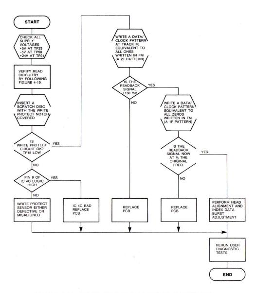
FIGURE 4-23. WRITE CIRCUIT DIAGNOSTIC FLOWCHART
