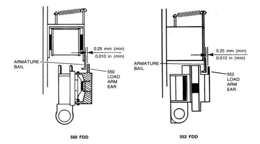
FIGURE 4-15. BAIL AND LOAD ARM CLEARANCE
