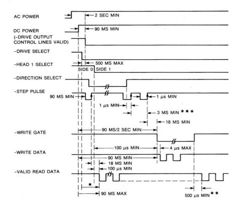
\* 35 MS MIN ELAPSE FROM HEAD LOAD START; OR, OPTIONALLY, A MINIMUM OF 15 MS ELAPSES IF STEPPER MOTOR POWER IS SWITCHED FROM LOWER POWER (+5 VDC) TO HIGH POWER (+24 VDC) INDEPENDENT OF HEAD LOAD.
