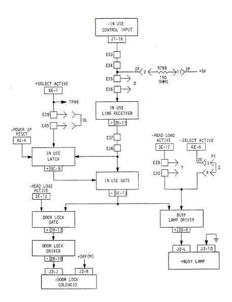
FIGURE 6-2. IN USE, DOOR LOCK AND BUSY LAMP FUNCTIONS
