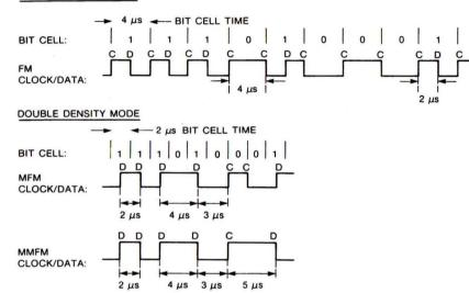
PULSE SEPARATION FORMAT FM: 1F, 2F (I.E., 4 μs, RESPECTIVELY) MFM: 1F, 3/2F, 2F (I.E., 4 μs, 3 μs, 2 μs, RESPECTIVELY) MMFM: 4/5F, 1F, 3/2F, 2F (I.E., 5 μs, 4 μs, 3 μs, 2 μs, RESPECTIVELY)
